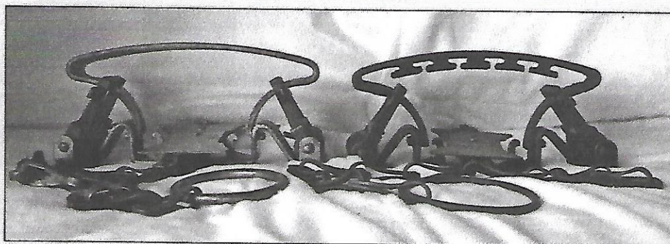
Triumph Master Grip Traps are very sought after because of their unique jaw configuration. The Triple Clutch feature was added to some of the traps. They are the added grippers below the jaws. Only about 1,000 of these traps were ever made, and they can sell for $500.
